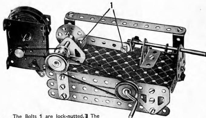
The Bolts 1 are lock-nutted. The Angle Brackets representing the piston are clamped to the Rod by a Nut and Bolt fastened in their elongated holes.
