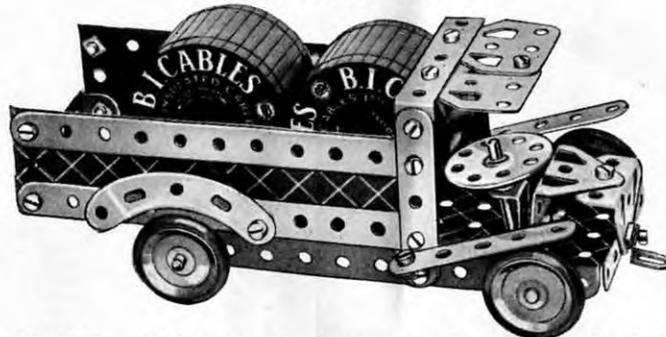
The  $2\frac{1}{2}''$  Curved Strips representing the rear mudguards are each fastened to the sides by a  $\frac{3}{8}''$  Bolt and Nut, with a Spring Clip between the mudguards and the  $5\frac{1}{2}''$  Strip to form a distance piece.
