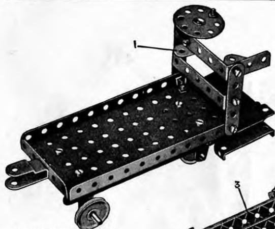
The steering wheel, a Bush Wheel, is secured to Reversed Angle Bracket 1 by means of a  $\frac{3}{8}$ " Bolt. Fig. 1.M45a shows how the *Magic Motor* is mounted to drive the front wheels. The front wheel axle is journalled in two Flat Brackets bolted to the  $5\frac{1}{2}$ " Strips 2 and 3.
