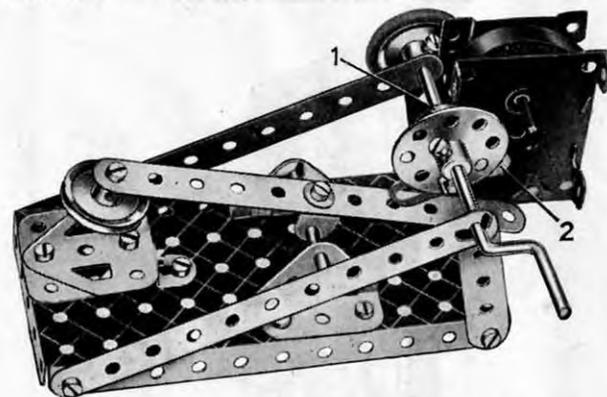
The  $\frac{1}{2}$ " fast Pulley 1 is driven from the pulley 2 on the *Magic Motor* by the Driving Band supplied with the Motor.
