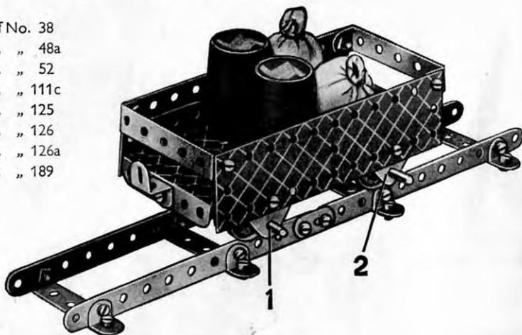
The axle bearings 1 are Flat Trunnions, and Trunnions 2, which fit underneath the Flanged Plate in the manner shown in the underneath view of the model Side Tipping Wagon (1.M46).
