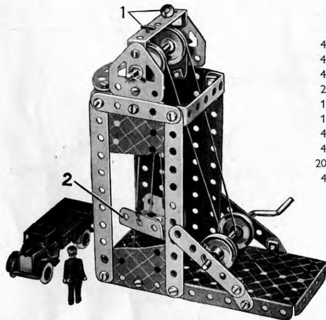
A Cord is taken from each side of the lift cage over the 1" Pulleys and secured to each end of the Crank Handle. The Cords must both be the same length otherwise the lift will tilt.
