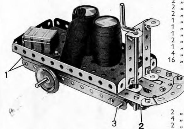
The two 5½" Strips 1 are fastened to the Flanged Plate by two Trunnions secured to the Plate on the underneath side. A Bush Wheel 2 is fixed on the Axle Rod 3, which passes through the end holes of the 5½" Strips that form the sides of the truck frame.
