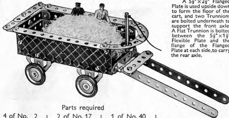
A  $5\frac{1}{2}'' \times 2\frac{1}{2}''$  Flanged Plate is used upside down to form the floor of the cart, and two Trunnions are bolted underneath to support the front axle. A Flat Trunnion is bolted between the  $5\frac{1}{2}'' \times 1\frac{1}{2}''$  Flexible Plate and the flange of the Flanged Plate at each side, to carry the rear axle.
