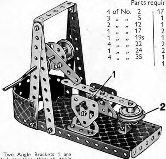
Two Angle Brackets 1 are bolted together through their holes and also are bolted to two 2½" Strips to form a double bracket. The 1" fast Pulley 2 is fitted with a 1" Rubber Ring.
