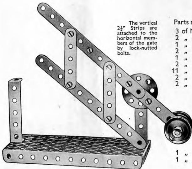
The vertical 2½" Strips are attached to the horizontal members of the gate by lock-nutted bolts.
