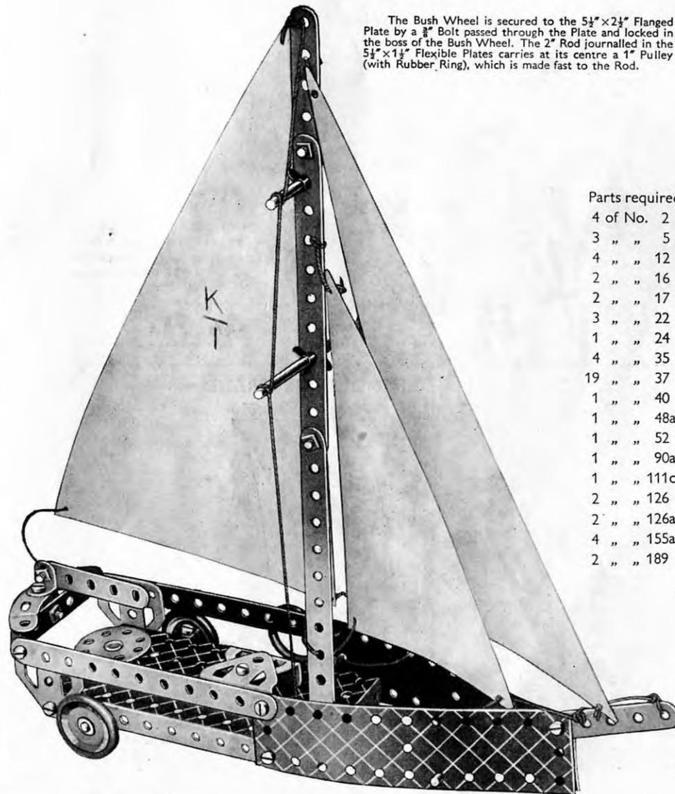
The Bush Wheel is secured to the  $5\frac{1}{2}$ " x  $2\frac{1}{2}$ " Flanged Plate by a  $\frac{3}{8}$ " Bolt passed through the Plate and locked in the boss of the Bush Wheel. The 2" Rod journalled in the  $5\frac{1}{2}$ " x  $1\frac{1}{2}$ " Flexible Plates carries at its centre a 1" Pulley (with Rubber Ring), which is made fast to the Rod.
