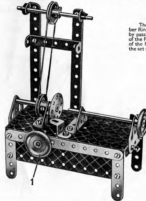
The 1" fast Pulley with Rubber Ring 1 is secured to the Strip by passing a Bolt from the inside of the Flexible Plate into the boss of the Pulley and then tightening the set screw.
