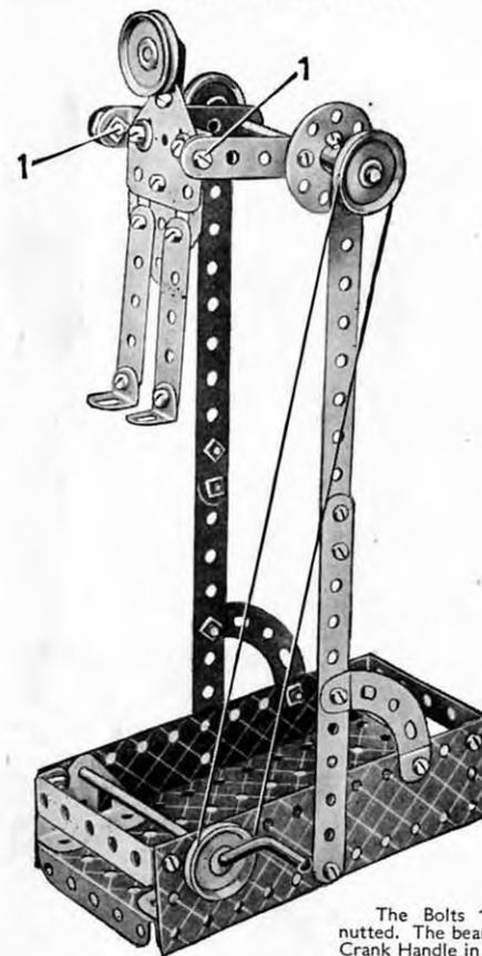
The Bolts 1 are lock-nutted. The bearings for the Crank Handle in the Flexible Plates are reinforced by Trunnions bolted to the Flanged Plate.
