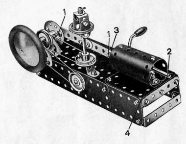
The bearings for the Rod representing the crankshaft are a Flat Trunnion and a Trunnion. The crankshaft carries a Road Wheel and a 1" Pulley at one end, a second 1" Pulley between the bearings, a and Bush Wheel at its other end.
