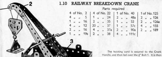
Handle, and then led over the §" Bolt 1. It is then passed through the pulley block and fastened to the jib at 2. The jib is attached to the Bush Wheel 3 by means of Angle Brackets and the complete unit is pivoted as follows. A §" Bolt is passed through the  $5\frac{1}{2}$ "  $\times 2\frac{1}{2}$ " Flanged Plate from the underside, and is secured in the boss of the Bush Wheel by its set screw.
