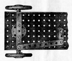
S.M.162 The simple steering gear will be found suitable for most small model vehicles.
