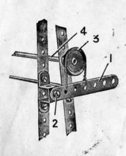
S.M.111. The brake lever consists of a  $3\frac{1}{2}$ " Strip 1, pivotally attached at a suitable point on the frame of the model to be fitted, by means of a lock-nutted  $\frac{3}{8}$ " Bolt 2. The driven shaft 4 is fitted at one end with a 1" fast Pulley 3 round which a short length of cord is passed. The two ends of this Cord are secured to the brake lever at the points shown in the illustration.
