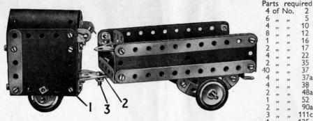
Each side of the tractor unit consists of a 24" x 24" Flexible Plate bolted to a Double Angle Strip 1. A  $4\frac{1}{2}'' \times 2\frac{1}{2}'''$  Flexible Plate is curved and attached to each side to form the top. The front and rear of the unit are each filled by a  $2\frac{1}{2}i'' \times 1\frac{1}{2}i'''$  Flexible Plate and a Flat Trunnion. The front axle is mounted in two Fishplates.
