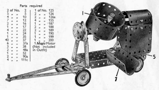
The model is built up on a Flanged Plate. The front axle is journalled in a Double Angle Strip lock-nutted to a Trunnion bolted to the Plate. The rear axle runs in two Curved Strips.
