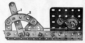
S.M.112. This mechanism is a form of band brake in which the lever 1 can be held in any position by means of the quadrant 2. In this way varying pressures can be applied to the Pulley forming the brake drum.
