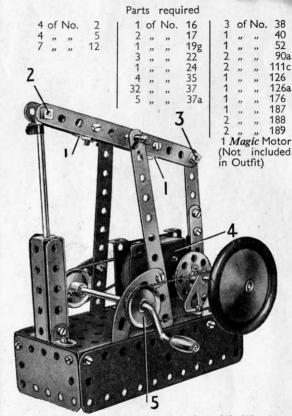
The engine bed or base consists of two  $5\frac{1}{2}''\times1\frac{1}{2}''$  and two  $2\frac{1}{2}''\times1\frac{1}{2}''$  Flexible Plates bolted to the sides of a Flanged Plate. Two  $5\frac{1}{2}''$  Strips form the supports for the beam, which pivots on a 2" Rod held in position by Spring Clips.
