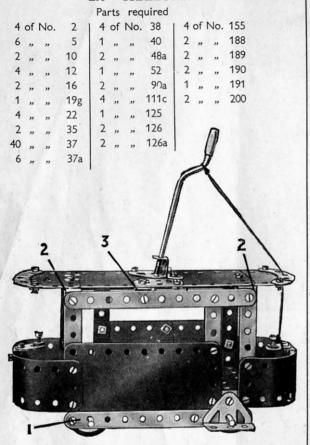
Two  $5\frac{1}{2}$ "  $\times 1\frac{1}{2}$ " Flexible Plates are curved and bolted across the ends of a Flanged Plate to form the driving compartments at each end, and a 4½" × 2½" Flexible Plate is used for one side of the model. This also is bolted to the Flanged Plate. The other side consists of two 1#" radius Curved Plates, flattened and bolted in position. Both sides are strengthened by a 5#" Strip, one of which is seen at 1: ..
