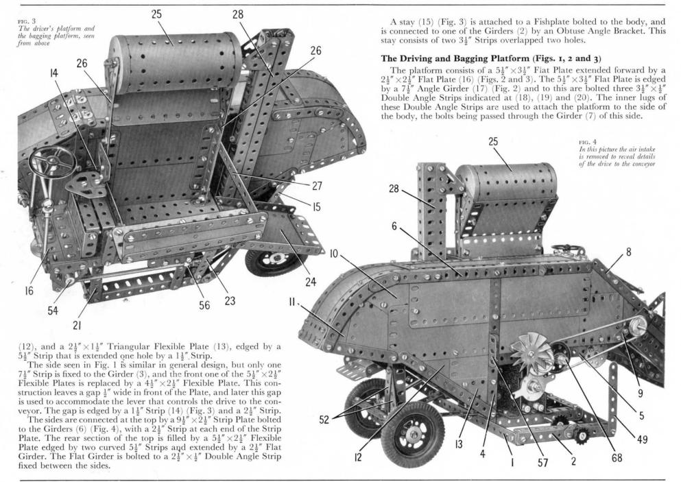
A built-up strip (21) (Fig. 3), made from two 2" Strips overlapped two holes, is bolted to one of the Girders (2) (Fig. 2) and is connected to Double Angle Strip (19) by an Angle Bracket. A 3" Angle Girder (22) (Fig. 10) is fixed to one of the Girders (1) and is attached to the Double Angle Strip (19) by a  $\frac{1}{2}$ " Corner Angle Bracket (see Fig. 10). A  $3\frac{1}{2}$ " Strip (23) is secured to the Girder (17) and is connected to one of the Girders (2) by an Obtuse Angle Bracket.
