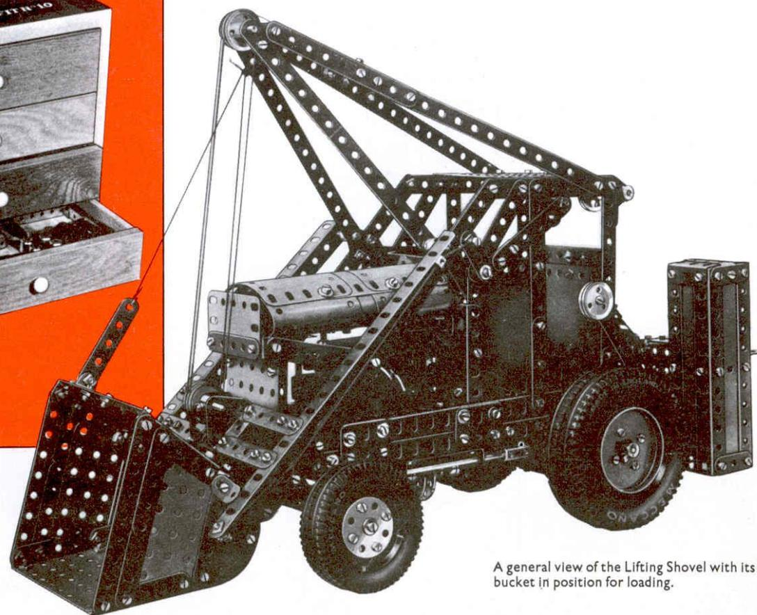
This striking model represents a popular type of mechanical lifting shovel used on large construction jobs where quantities of soil or other material have to be loaded into vehicles for removal from the site. Power is provided by a Meccano E15R Electric Motor that drives the road wheels through a differential. The lifting and unloading movements of the shovel are controlled from the cab, and the hoisting winch is fitted with an automatic brake.
