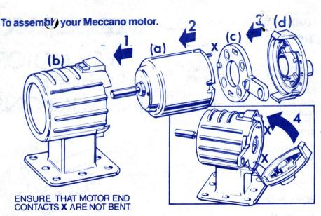
Position motor (a) in motor housing (b) with end contacts at top and bottom (see inset). Locate the switch lever (c) (smooth side outwards) over the motor end contacts. Hold the motor end cap (d) with 'Meccano' upwards. Insert the lower locating lugs then position top locating lug and push until it 'clicks' home.
