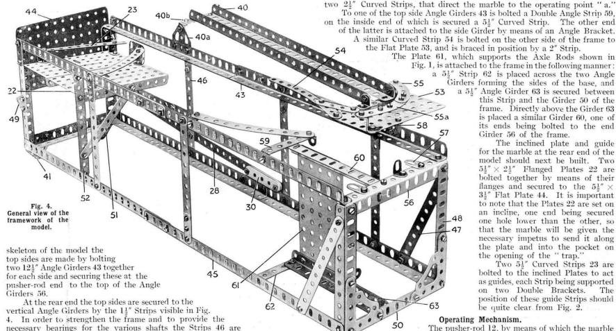
its ends being bolted to the end Girder 56 of the frame. The inclined plate and guide for the marble at the rear end of the model should next be built. Two  $5\frac{1}{2}'' \times 2\frac{1}{2}''$  Flanged Plates 22 are bolted together by means of their flanges and secured to the  $51'' \times$ 3½" Flat Plate 44. It is important to note that the Plates 22 are set on an incline, one end being secured
