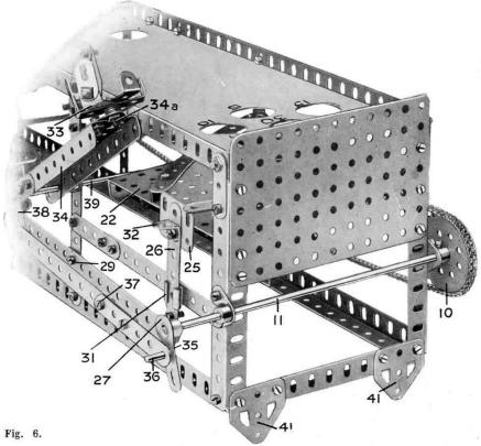
End view of the Bagatelle Table, showing stop plate mechanism, etc.
