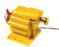
3-12 volt DC motor with 6-ratio gearbox. super-efficient, precision made reversible motor with low current consumption. The motor works from a 3 to 12 volt DC power source as supplied by suitable battery or series of batteries.
