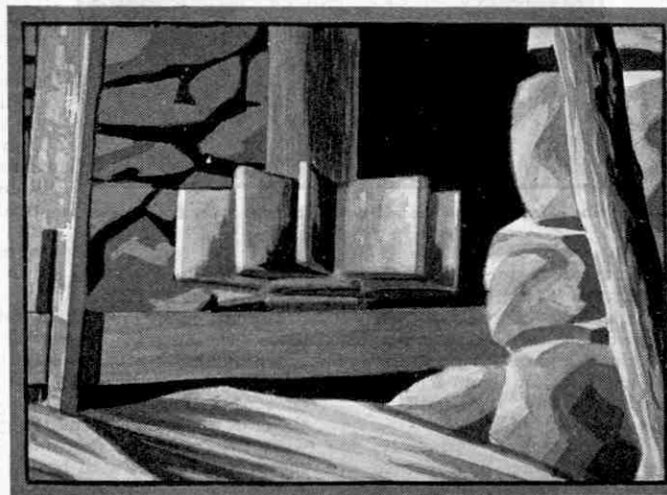
Closer view of paddles and shaft of a Norse Mill
