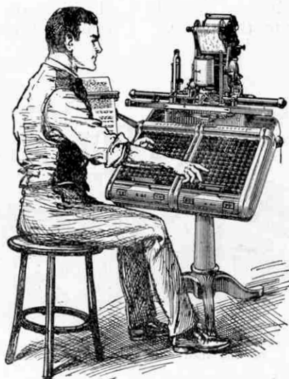
At work on the Monotype Keyboard. As the keys are depressed holes are punched in the paper ribbon on top of the machine. From "Remarkable Machinery," by courtesy of the publishers, G. G. Harrap & Co. Ltd.
