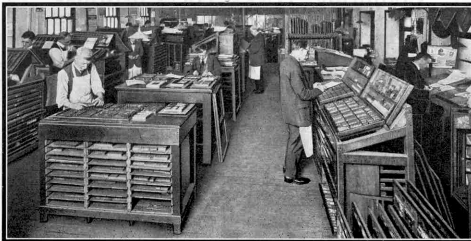
Where type is composed by hand. The sloping boxes divided into compartments are cases containing types
