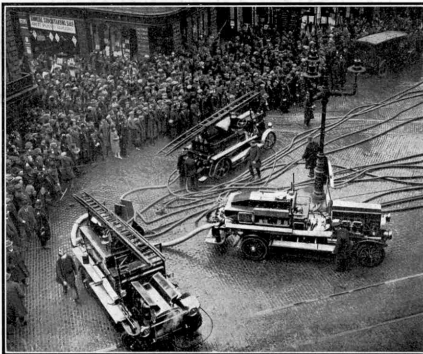
The scene at a large fire at Nottingham. The suction hose leading from a street main to the engine in the background is clearly shown. Note the several unconnected lengths of hose laid out in reserve
