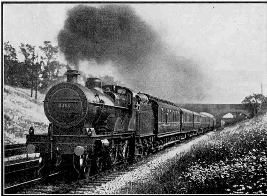
One of the "25's" at full speed, near Mill Hill. As will be seen, the Standard Compound Locomotive No. 1100 was fitted as an oil burner. This was done for experimental purposes, and the apparatus has since been removed
