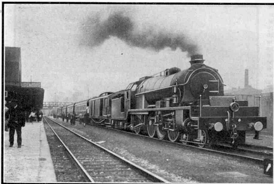
[C. J. Allen] The "Edelweiss Pullman" at Luxembourg. It is headed by one of the monster 4-cylinder "Pacifics" of the Belgian National Railways, and about to begin the non-stop journey of 102½ miles through the Ardennes to Namur
