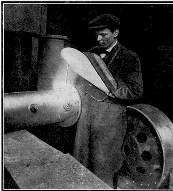
Welding flange on a steel pipe 12 in. in diameter. Our illustration shows that the heat of the electric arc is concentrated in a very small space
