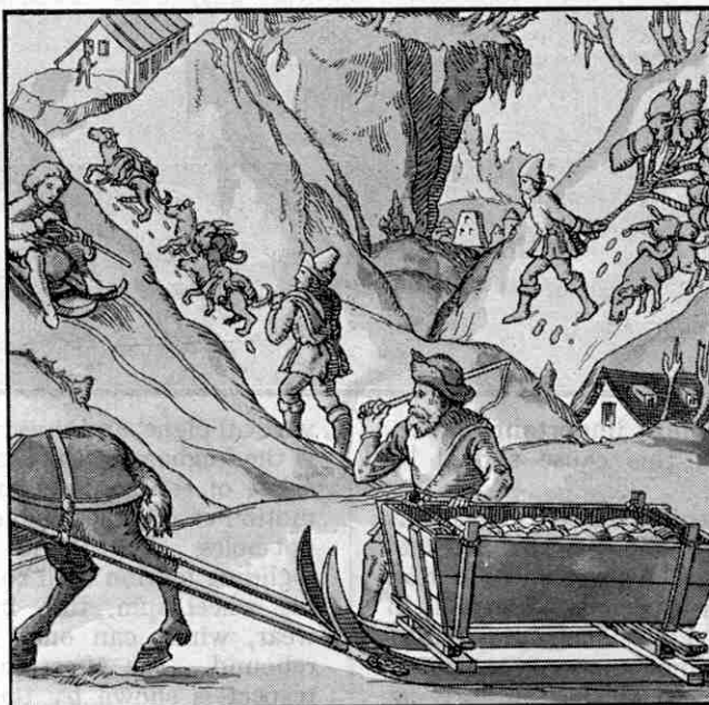
From an old engraving Removing ore, showing box carried on sledge and dogs with pack saddles.
