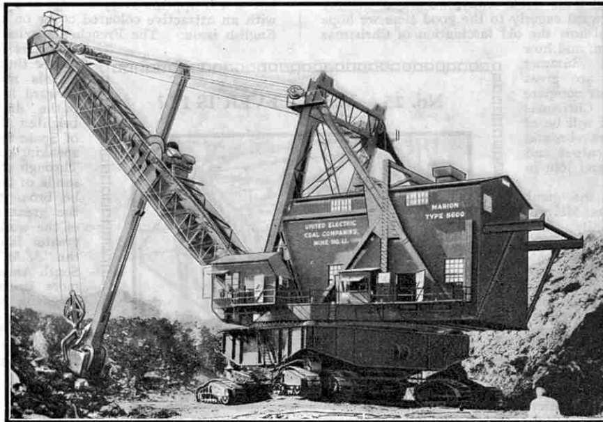
The world's largest shovel stripping the overburden from coal in the open pit mine at Du Quoin, in the United States. The electrically operated scoop is capable of lifting 16 tons of coal. For this and the illustrations on the opposite page we are indebted to the International General Electric Company.
