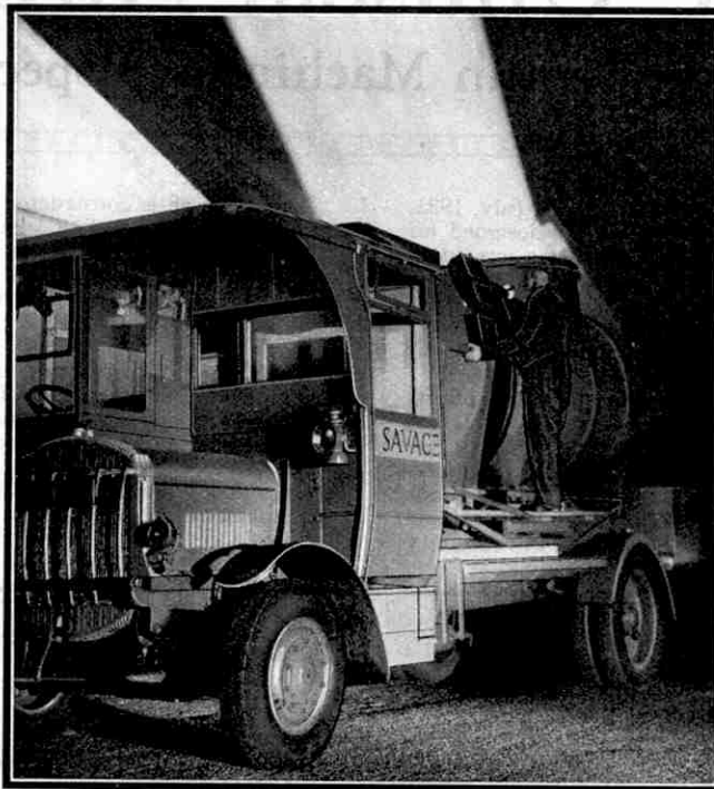
The Savage searchlight mounted on a petrol-electric chassis from which the necessary current is obtained. The movements of the beam may be controlled from a distant point by means of remote control apparatus.
