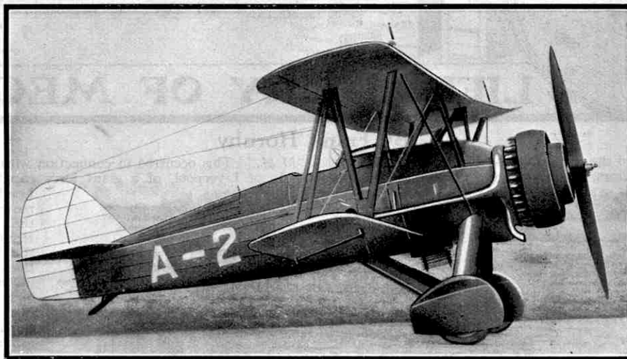
The A.W.XVI single-seater fighter, equipped with an Armstrong Siddeley "Panther" engine. This machine, which has a speed of 200 m.p.h. at a height of 15,000 ft., was described on page 715 of the "M.M." for September, 1931. Our photograph is published by courtesy of Sir W. G. Armstrong Whitworth Aircraft Co. Ltd.
