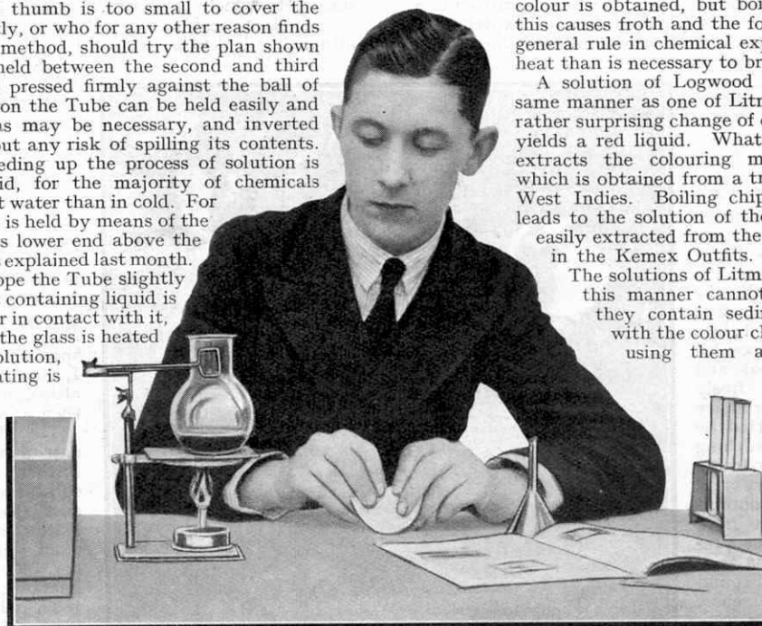
Fig. 2. Making a solution of Litmus in readiness for the preparation of test papers. A Filter Paper is being folded while the Litmus is heated with water.
