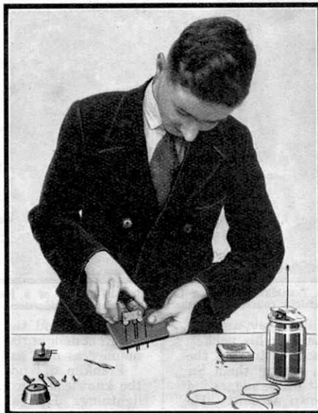
Another stage in building the Bell, showing the complete electro-magnet being placed in position.
