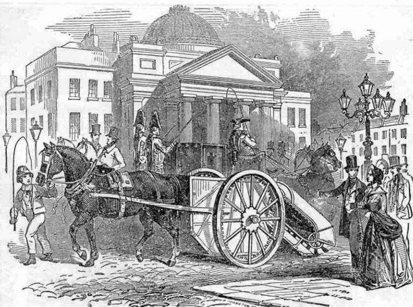
Whitworth's Mechanical Road Sweeper in operation at Manchester about 1851-2.
