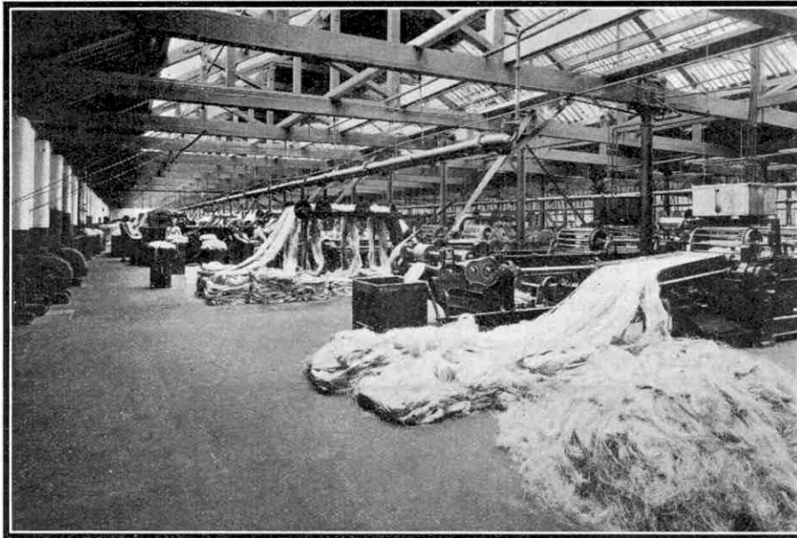
A preliminary stage in rope making; fibre-preparing machinery at work. The photographs illustrating this article were taken at the extensive Belfast Ropeworks.
