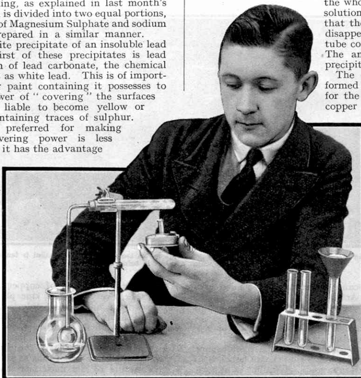
Fig. 1. Precipitating salt from solution by passing hydrochloric acid gas into it. The salt is obtained in a pure form that does not become damp when exposed to moist air.
