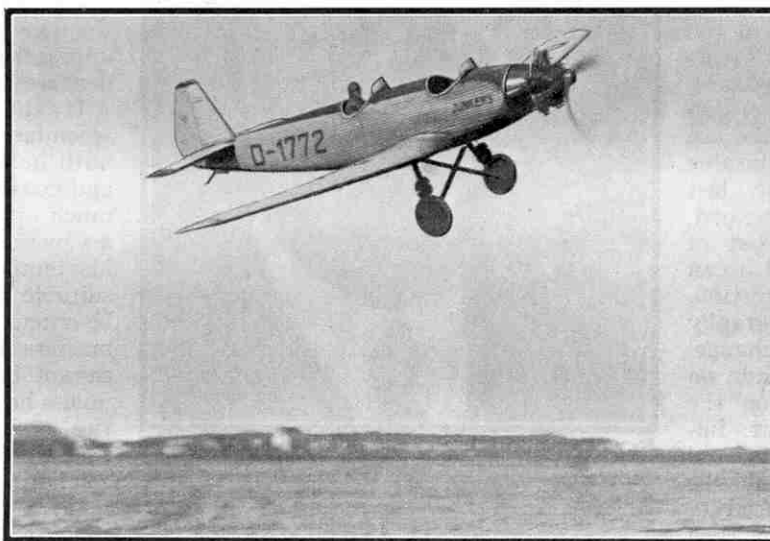
A Junkers "Junior" all-metal light aeroplane in flight. The familiar Junkers practice of employing corrugated metal can be seen in this illustration. Photograph by courtesy of Junkers-Flugzeugwerke, A. G.
