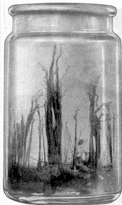
Fig. 2. A Chemical Garden grown by placing crystals of Cobalt Nitrate in a solution of water glass.
