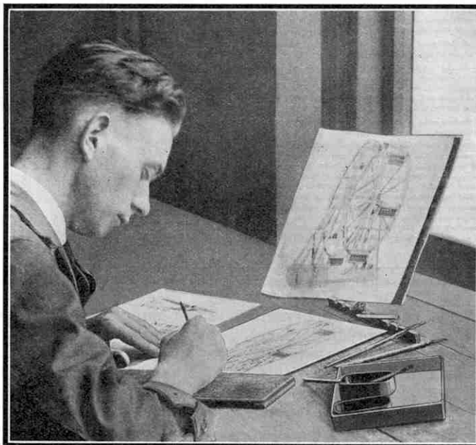
One of the final processes. Parts of the plate are being covered with protective material before it is returned to the etching machine.
