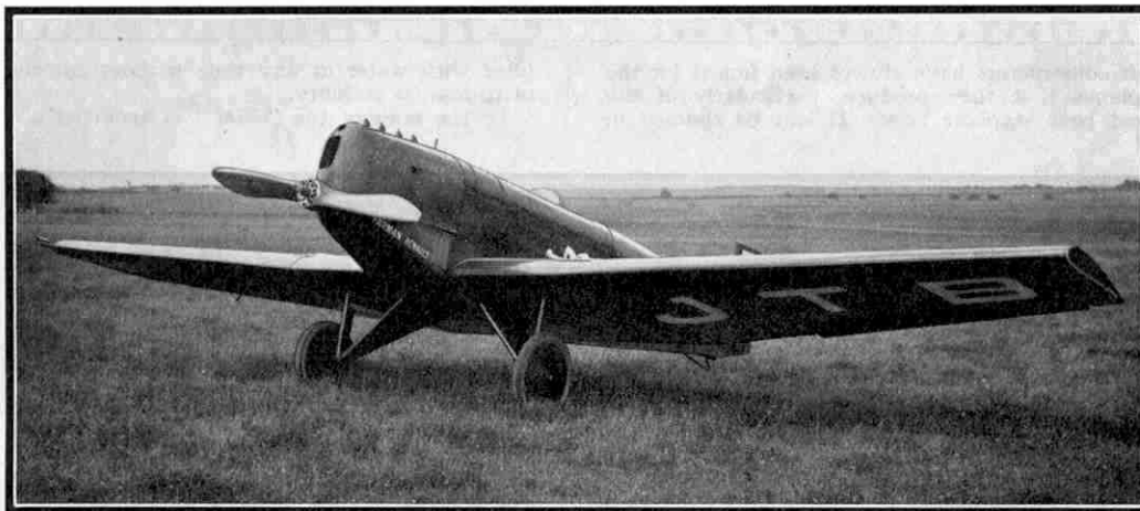
A three-quarter front view of the Farman F-231 low wing monoplane which is equipped with a Renault engine and has a top speed of 118 m.p.h. For this photograph we are indebted to Avions Henri et Maurice Farman.
