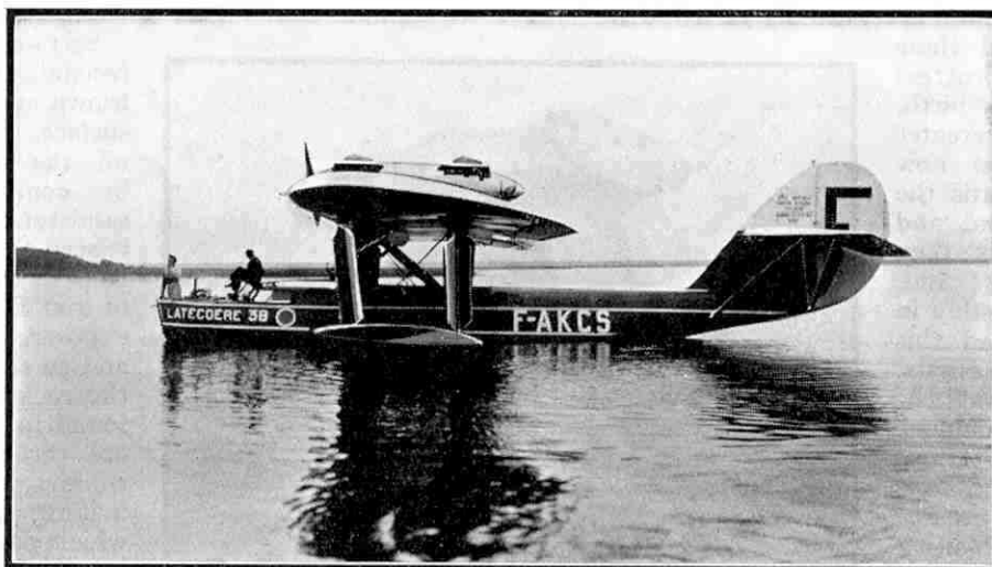
This illustration, published by courtesy of Société Industrielle d'Aviation Latécoère, shows the Latécoère 38-0, a twin-engined postal flying boat popular with French air line companies.
