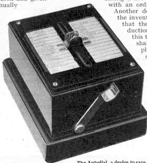
The Autodial, a device to save time and trouble in using an automatic telephone. The photographs on this page are reproduced by courtesy of Dictograph Telephones Ltd.
