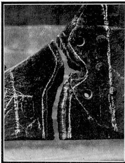
The damaged stern-frame of the "Lafian" prepared for welding by cutting along the line of fracture by means of an oxy-acetylene torch.
