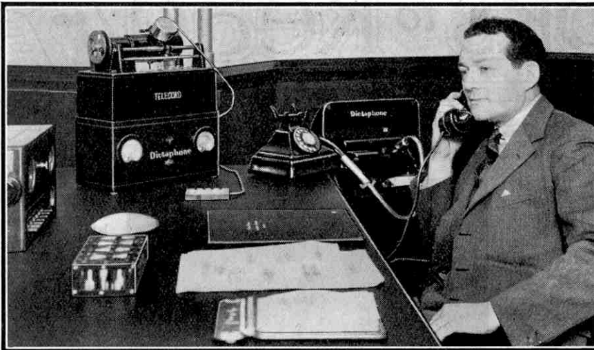
The Telecord in use for making a permanent Dictaphone record of a telephone conversation. If desired, only the incoming message is recorded. Photograph by courtesy of the Dictaphone Company Ltd.
