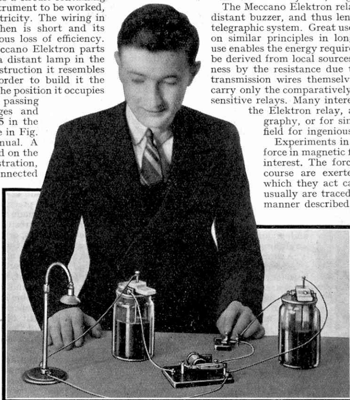
A Meccano Elektron relay in use for distant control of an Elektron electric lamp. The construction of the relay is described in the accompanying article.
