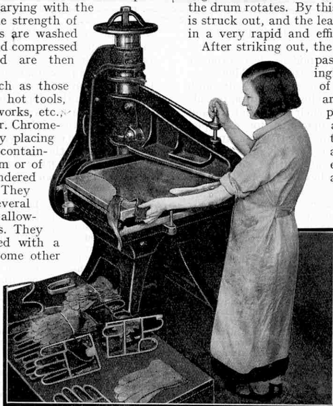
Cutting out glove parts on a power stamping machine. The peculiar knives or webbs used on the machine can be seen in the lower left-hand corner of the illustration.
