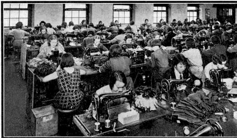
A view of the sewing room where the separate pieces of leather are sewn together by power driven machines.
