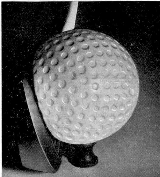
A photograph, taken with an exposure of one five-thousandth of a second, showing that one side of a golf ball is flattened when struck by a club. (See below.)
