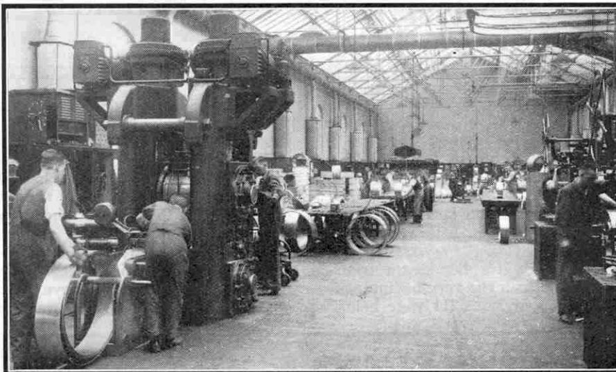
Fig. 3. Rolling-stainless steel strip for aircraft manufacture.
