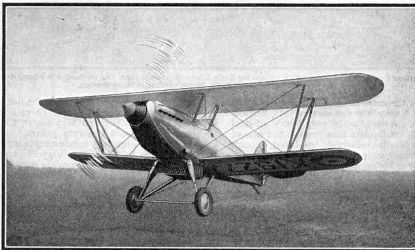
The Hawker "Fury" single-seater interceptor fighter. It has a top speed of 240 m.p.h. Photograph courtesy of Hawker Engineering Co. Ltd.
