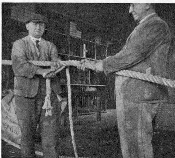
Splicing cotton driving ropes. The splice used takes 9 ft. to 15 ft. of rope.
