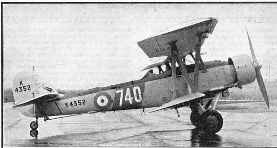
Broadside view of the Blackburn "Shark" Coastal Protection aeroplane. There is also a seaplane version of this machine.
