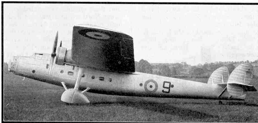
This broadside view of the Bristol 130 Transport-Bomber gives a good idea of the great depth of the fuselage and breadth of the wings. When used as a troop carrier the machine can convey 24 soldiers with complete equipment. Photograph by courtesy of The Bristol Aeroplane Co. Ltd.
