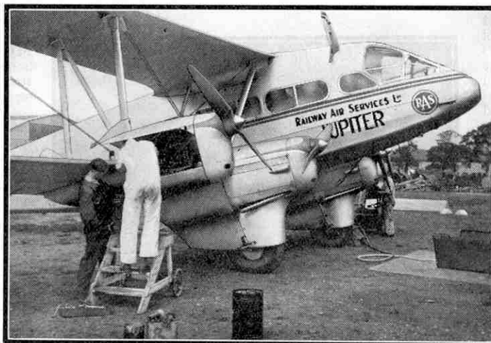
Overhauling one of the engines of "Jupiter," a de Havilland D.H.86 air liner of Railway Air Services, by whose courtesy the photograph is reproduced.
