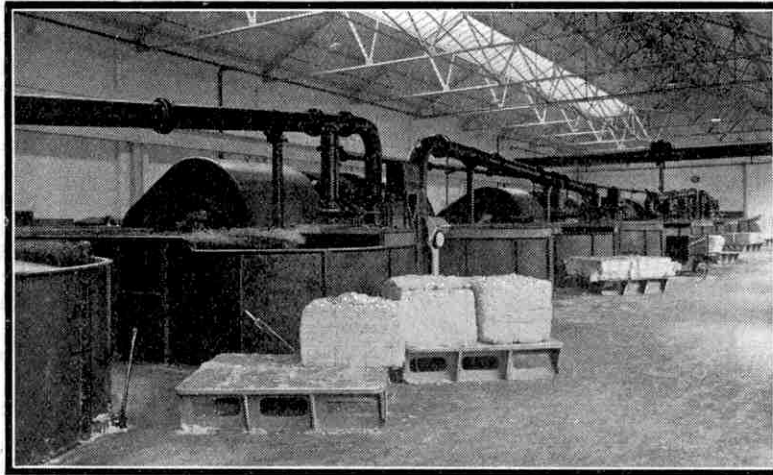
Wood pulp in the breaker house, in which it is broken up by beating in water. At the top of the page is a panoramic view of the works at Ellesmere Port, Cheshire, of Bowater's Mersey Paper Mills Limited, to whom we are indebted for the illustrations to this article.
