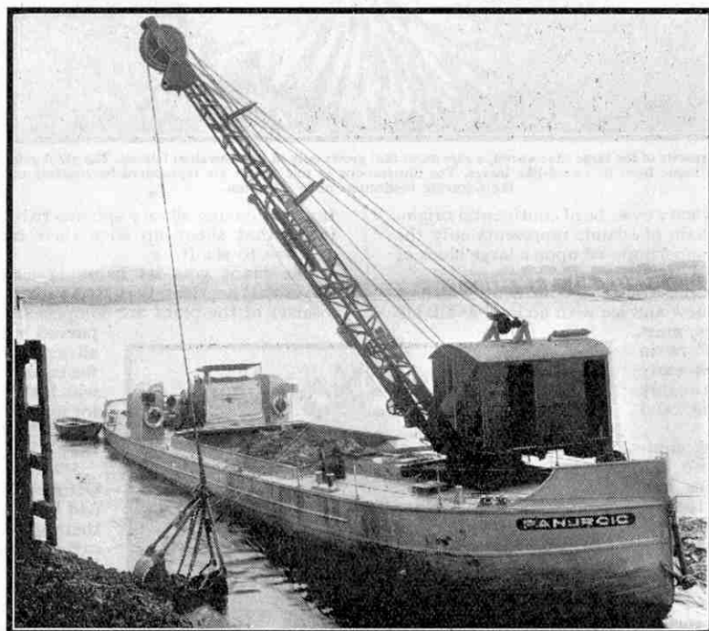
The dredger "Panurgic" at work in the River Trent. It is equipped with a Priestman Diesel-engined dredging crane. Photograph by courtesy of Priestman Bros. Ltd., Hull.
