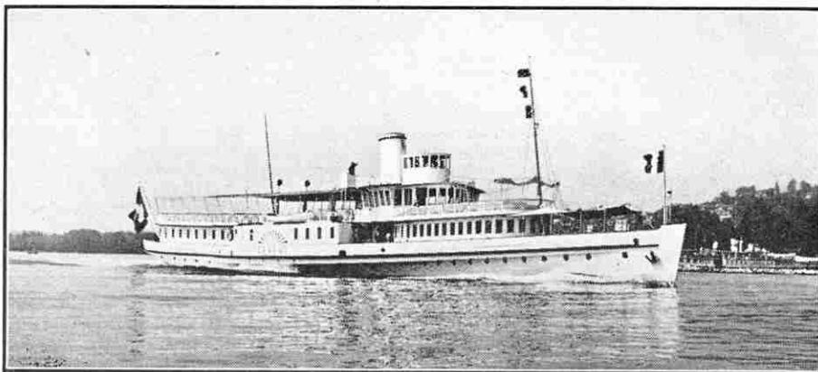
The paddle vessel "Genève" on Lake Geneva. As explained on this page, this vessel was converted from a steamer to a motorship. Photograph by courtesy of Sulzer Bros. (London) Ltd.
