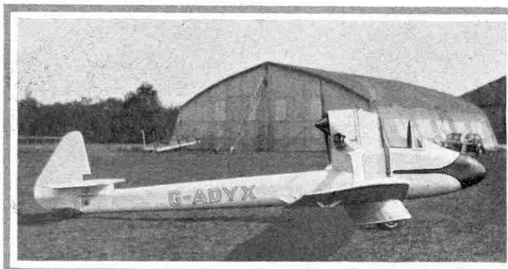
Two views of an unusual British lightweight, the Luton "Buzzard" single-seater "pusher" type monoplaner. Photographs by courtesy of Luton Aircraft Ltd.
