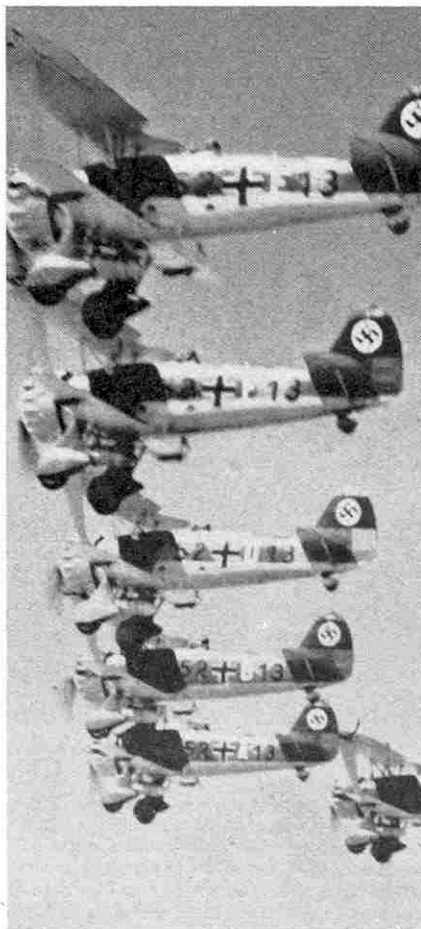
Henschel Hs 123 single-seater Dive-Bombers. This photograph and the lower one on the next page are reproduced by courtesy of "Flight."
