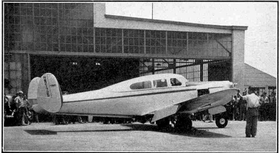
The new Vega "Starliner" transport aeroplane, in which the Menasco "Unitwin" engine is fitted. The photographs on this page are reproduced by courtesy of the Lockheed Aircraft Corporation, U.S.A.
