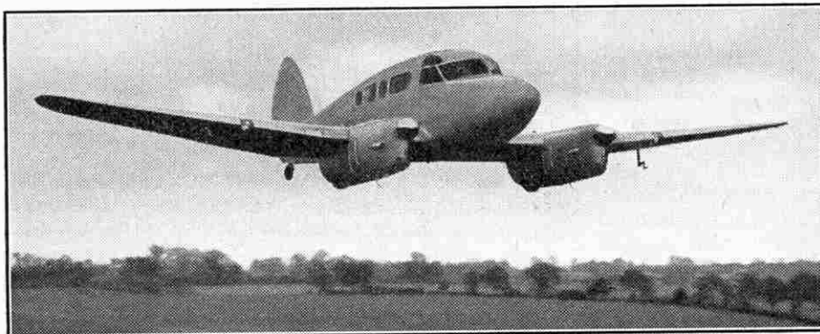
A Percival "Q" type monoplane in flight, with the undercarriage retracted into the rear of the deep engine nacelles. Photograph by courtesy of "The Aeroplane."
