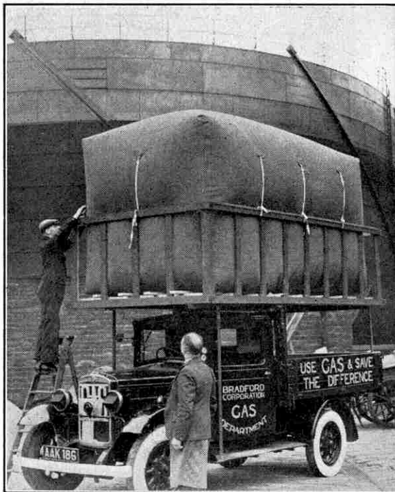
A motor lorry driven by coal gas. It was converted by the Bradford Corporation Gas Department, and the 432 cu. ft. of gas it can store in the envelope on the roof is equivalent to nearly two gallons of petrol.
