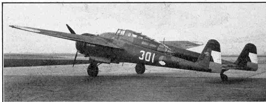
View of the Fokker G.1 fighter-bomber showing the short fuselage, and the two long, tapered booms that carry the wide tail unit. When fitted with "Bristol" Mercury VIII engines the G.1 can attain a top speed of 300 m.p.h. The photograph at the top of this page is reproduced by courtesy of N.V. Nederlandsche Vliegtuigenfabriek, Amsterdam.
