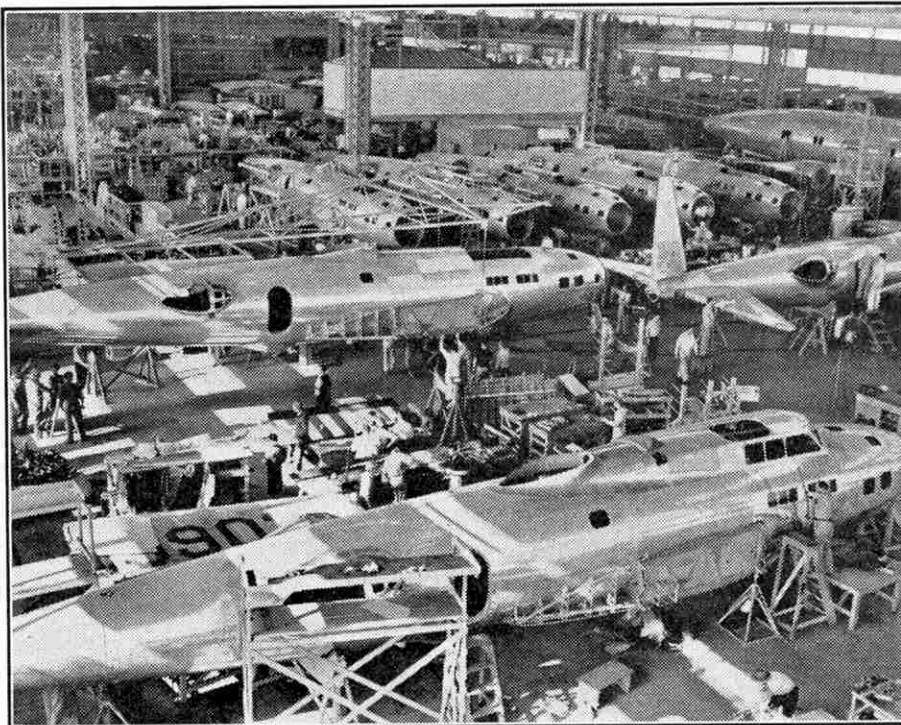
Boeing B-17B "Flying Fortress" Bombers under construction. The fuselages are shown at the start of the final assembly line, and the one in the centre of the picture is just being lowered by overhead cranes to its place on the assembly floor. Photograph by courtesy of Boeing Aircraft Company, U.S.A.
