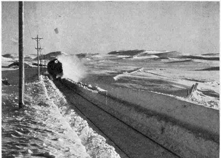
A striking winter scene on the Oslo-Bergen line, near Finse. The train is fitted with a snow plough.
