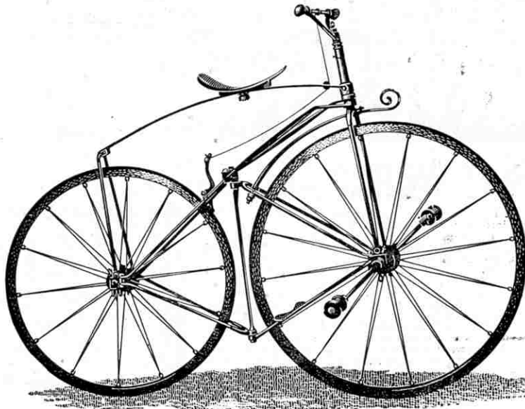
THE PHANTOM One of the first machines to be fitted with rubber tyres.
