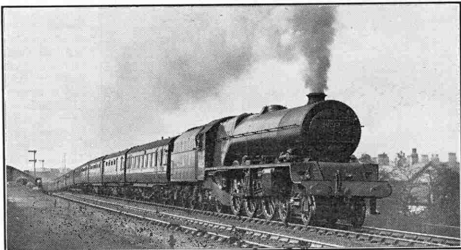
Liverpool-London express headed by 4-6-2 No. 6210 "Lady Patricia," one of the first series of L.M.S. "Pacifics."
