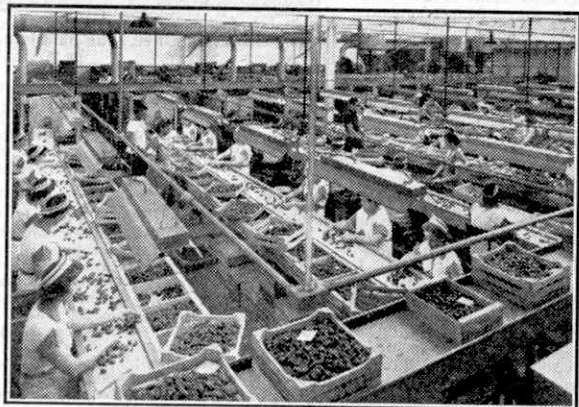
Grading dates. Trained graders select the fruit and sort it according to size, quality, texture and moisture content before it is packed.
