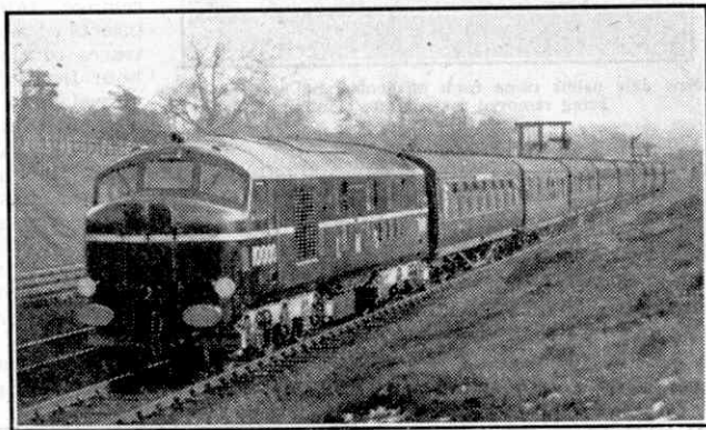
Britain's first diesel-electric express locomotive at work on the London Midland main line near Elstree. The train is the 2.15 Manchester express. Photograph by E. R. Wethersett.
