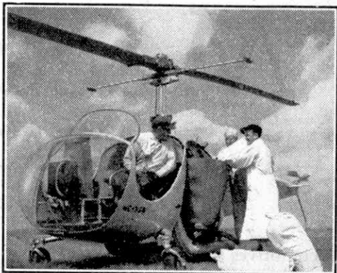
Loading agricultural dust into one of the two 220 lb. capacity hoppers of a Bell 47 crop-dusting helicopter.
