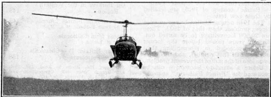
The helicopter in action. It can cover a 60 ft. swath in one pass, and dust between 100 and 200 acres an hour. The photographs on this page are reproduced by courtesy of Bell Aircraft Corporation, U.S.A.
