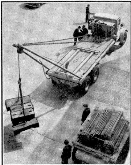
The self-loading oilfields truck can also act as a crane. The gin poles and other equipment needed are carried on the lorry and can quickly be assembled.
