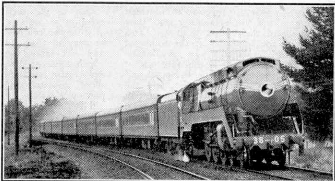
An air-conditioned express on the New South Wales Railways, Australia, hauled by "C.38" class 4-6-2 locomotive. Photograph by courtesy of the New South Wales Government Railways.
