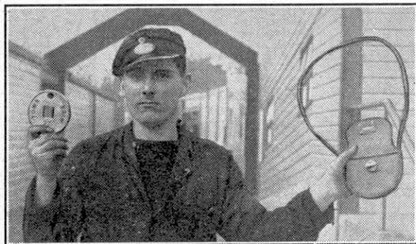
The fireman is holding a single line tablet in his right hand, while in the other he has the pouch, with hoop, in which it is carried.
