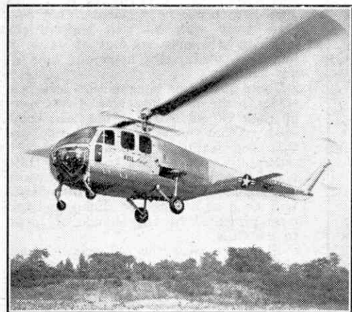
The Bell YH-12B military helicopter referred to on this page. Photograph by courtesy of Bell Aircraft Corporation, U.S.A.
