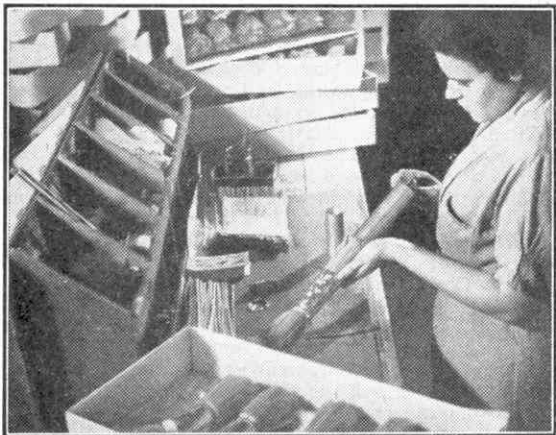
Crackers are formed round a metal cylinder, which is in two portions, and this illustration shows the second part of a cylinder being removed during the making of a cracker.
