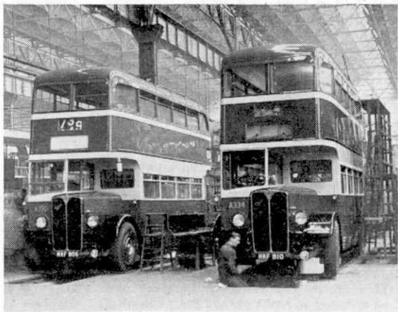
A scene in the L.C.P.T. depot in Edge Lane, showing two A.E.C. Regent Mk. III buses, with L.C.P.T. bodies on Weymann shells.
