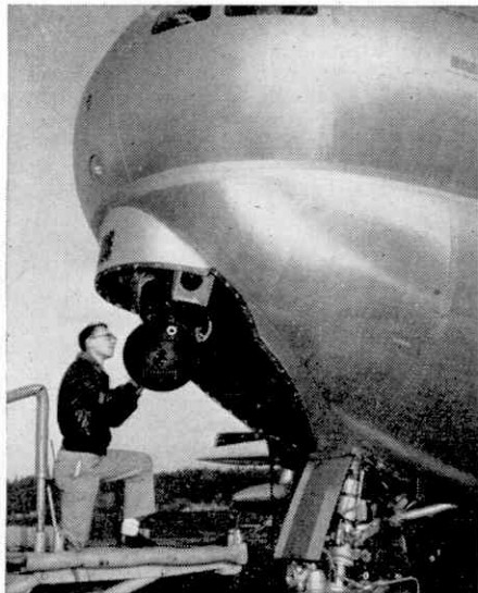
A Boeing electronics technician making final adjustments to the APS-42 radar antenna in the nose of a KC-97G Stratofreighter.
