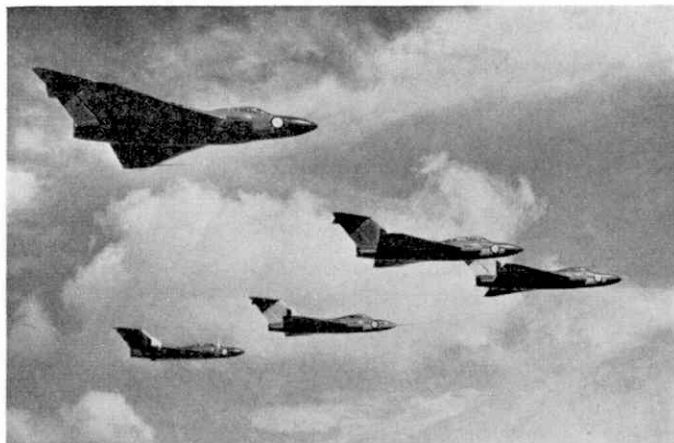
Javelin F. (A. W.) Mk. 1, the world's first twin-engined delta fighter.
