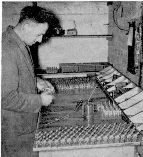
The assembly of engines for model aircraft in the works at Barnoldswick of Davies, Charlton Ltd., to whom we are indebted for our illustrations.
