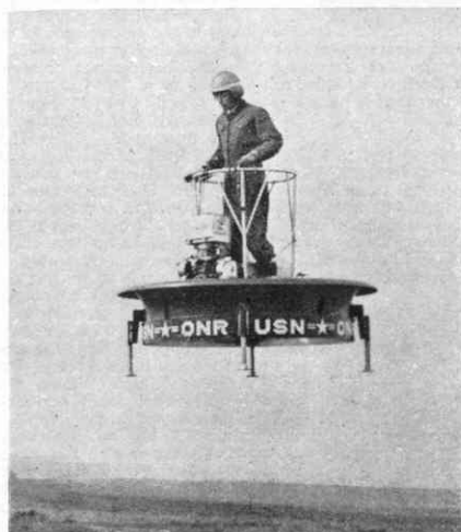
Literally a "Flying Platform," this Hiller research aircraft is claimed to be the simplest powered flying machine ever tested.
