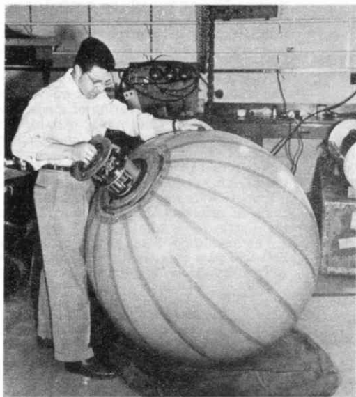
A nylon sphere containing a radio transmitter that was ejected from an Aerobee rocket at very high altitudes. The first satellites may be made in a similar manner, but will be smaller. University of Michigan photograph.
