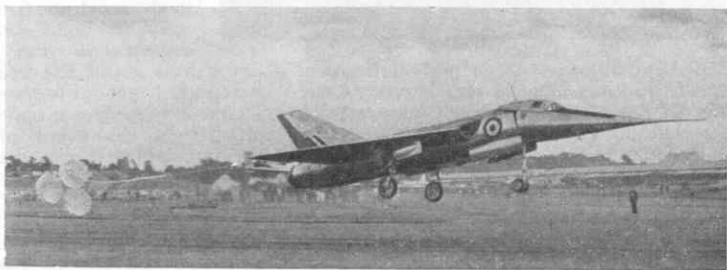
The Fairey F.D.2 turbojet-powered aircraft, with nose depressed and parachutes, acting as a brake, streaming behind, comes in to land at Farnborough. Photograph by courtesy of "Flight."
