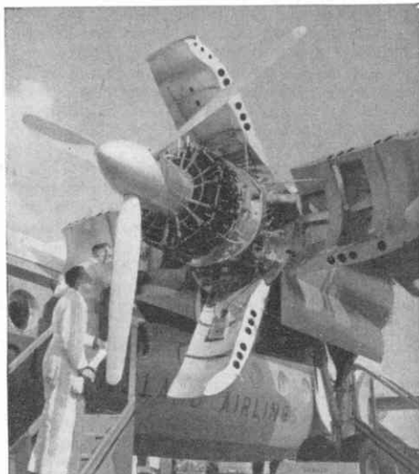
Handley Page Herald of the type ordered for Air Kruiise, showing the "petal" engine cowling open. A Shell photograph.
