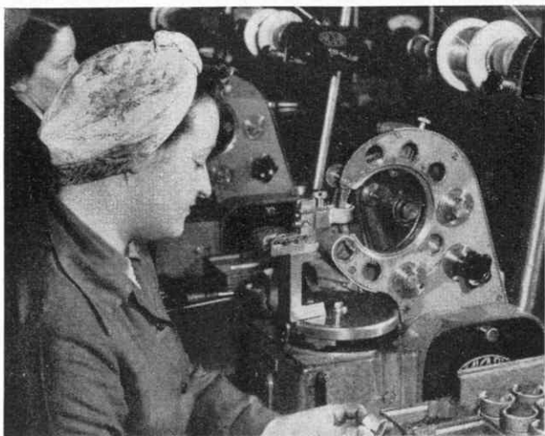
The ingenious machine on which the variable resistance is wound.
