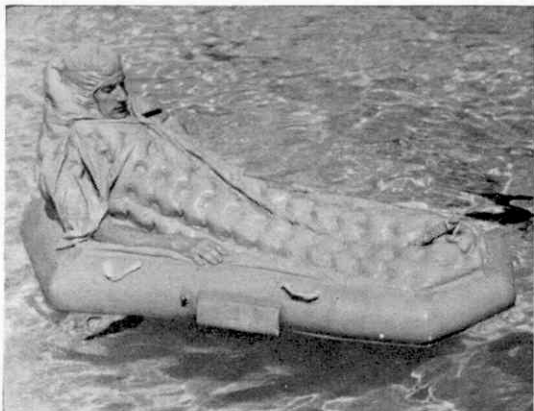
A victim of the sea in a single seat life-raft with an inflatable canopy for protection from exposure.
