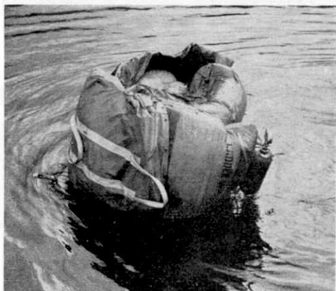
A life-raft dropped in the sea beginning to burst from its casing or valise on inflation.
