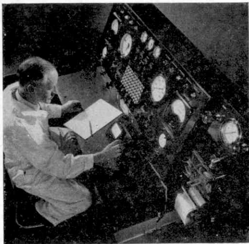
The control panel of a brake lining test machine in the new Ferodo Research Laboratories. Brake pressure, brake reaction torque pressure and lining temperature are recorded and a special counter gives stopping times to the nearest hundredth of a second.
