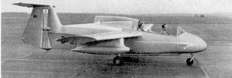
This unusual aircraft is the German-built RW3 Multoplane. The propeller is mounted in a slot between the fin and the rudder.
