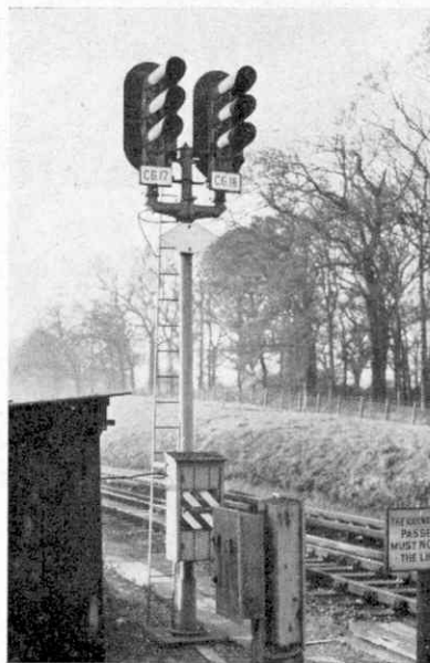
A colour light junction signal of the three-aspect type at Wivelsfield, Sussex. B.R. Southern Region Official photograph.
