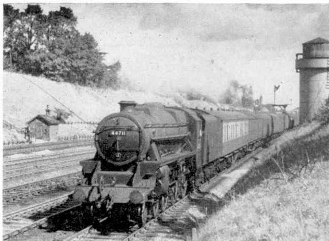
L.M.R. class 5 4-6-0 No. 44711 on an up train of empty stock near Bushey. Photograph by G. R. Mortimer.
