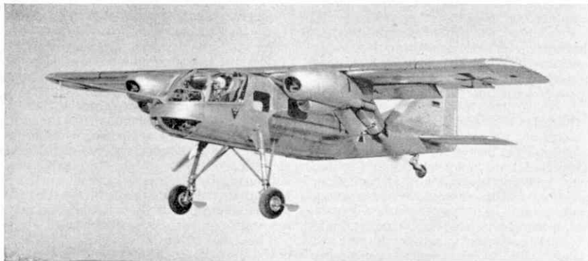
Intended for research—the Dornier Do 29 seen in flight with the pusher propellers and drive-shafts at the rear of the nacelles, tilted downwards.
