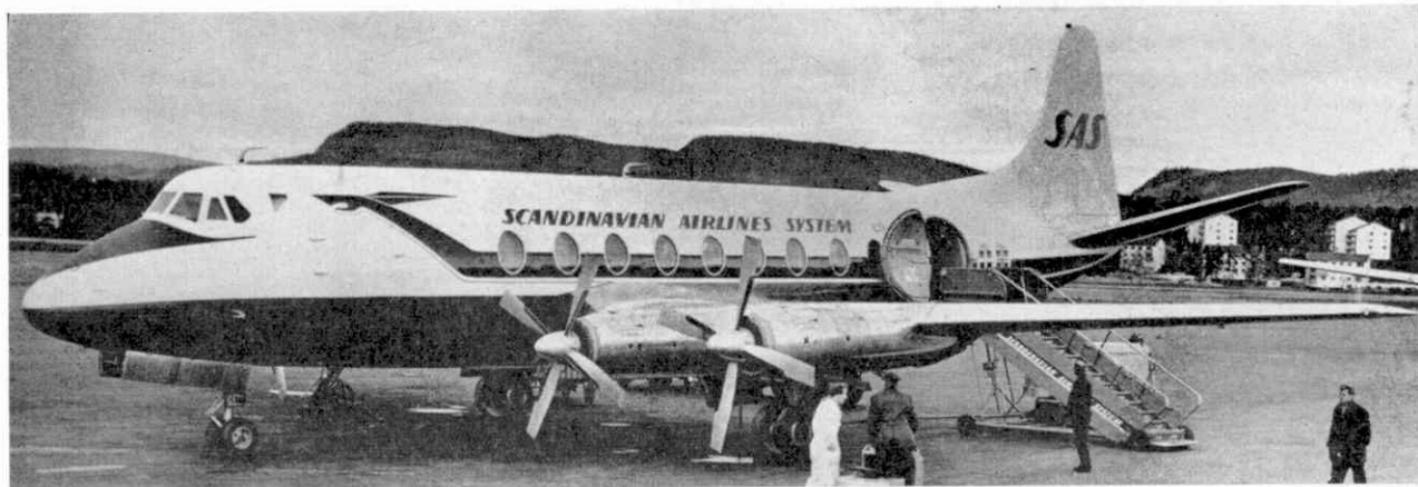
The forty-third airline to operate the Vickers Viscount turboprop airliner is SAS. The aircraft seen above is arranged as a 48-seater.
