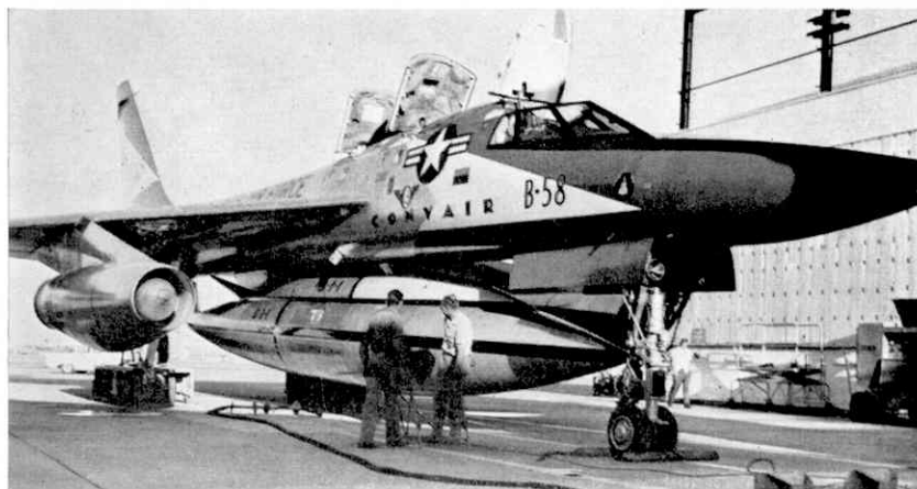
Two-part pod. Convair crew inspects the new two-part droppable pod on an Air Force B-58 Hustler bomber. The new pod, which provides additional speed and range, is in production at the Fort Worth, Texas, plant of Convair Division of General Dynamics Corporation, by whose courtesy this picture is reproduced.
