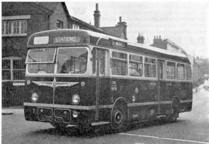
This Reading Corporation A.E.C. "Reliance" No. 7 (NDP 425) with a Burlingham standee-type body shows one modern trend in One-Man Operation in our bigger towns. Surfleet Transport photograph.
