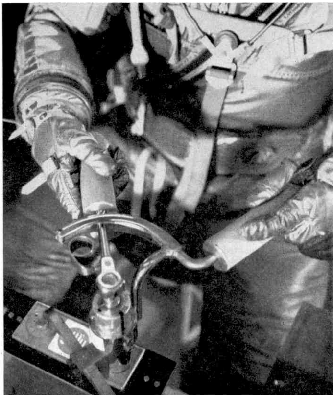
This nut and bolt tool for use in space has a reaction-less ratchet drive and a connection to the work-piece. Photograph by courtesy of the American Machine Foundry.
