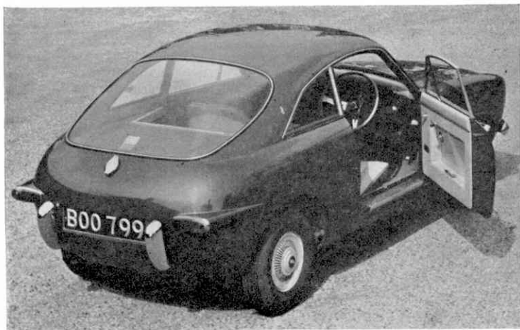
The Ogle Super SX 1000 based on the Mini-Cooper, has a top speed of 93 m.p.h. and very lively acceleration. It has twin beam headlamps and a 10½ gallon fuel tank.
