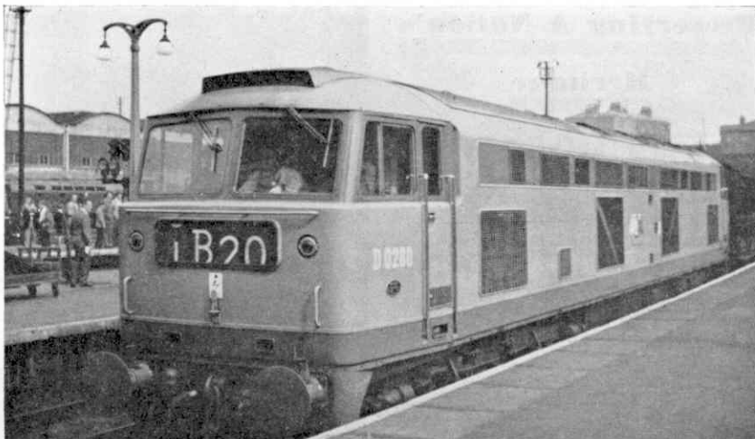
Another illustration by J. Wyndham—the experimental Brush "Falcon" D.0280, hauling the "Master Cutler", draws into King's Cross.
