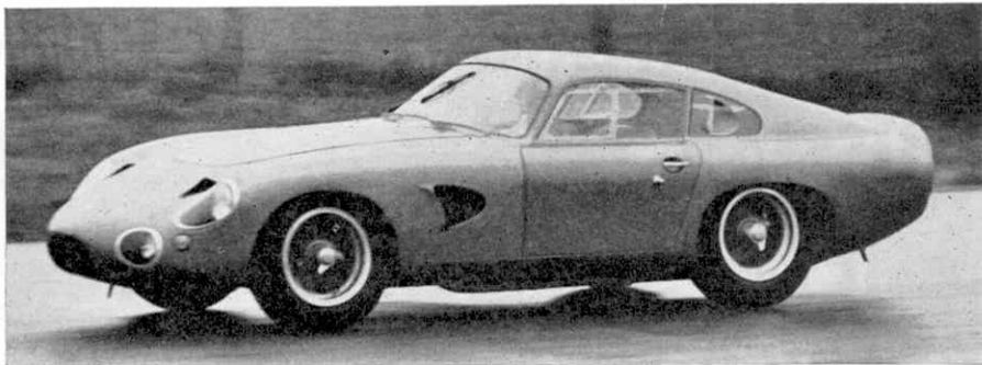
The Aston Martin Project 215 which made one that impression in the early laps at Le Mans but suffered later from transmission trouble. The flat, cut off tail makes an enormous difference to stability at speed and was suggested by B.R.M. driver Ritchie Ginther.
