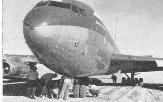
Above and Below: A Boeing 707 tests a new undercarriage assembly for landing the C-5A on unmade landing strips.
