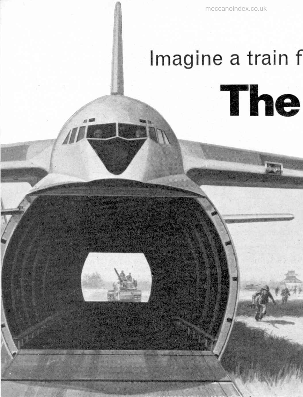
Loading of the huge C-5A will be through front and rear openings in the 40 yard long fuselage.
