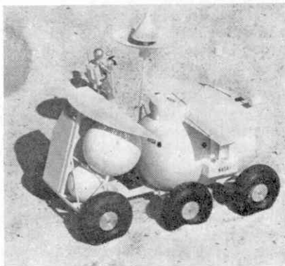
Above: a scale model of a mobile lunar laboratory (MOLAB). This would be the astronauts' 'mobile home' during a fortnight's stay on the lunar surface.
