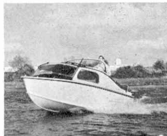
On the cover: The high performance Dolphin 16 Day Boat, built by Brooklands Aviation Ltd. at Northampton, uses outboard power up to 70 h.p.—top speed 27 knots. Photo: Brooklands Aviation Ltd., Marine Division.
