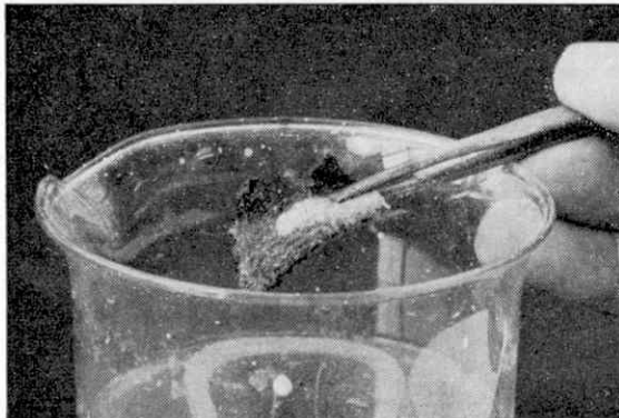
At left, top, man-made fibres (nylon and terylene) melt when heated. Natural fibres char and burn. This photo shows the terylene rope end (melted) and the natural fibre rope (charred). The treatment of a wool mixture fabric with acid, as shown in the beaker, dissolves the wool but leaves synthetic fibre intact.
