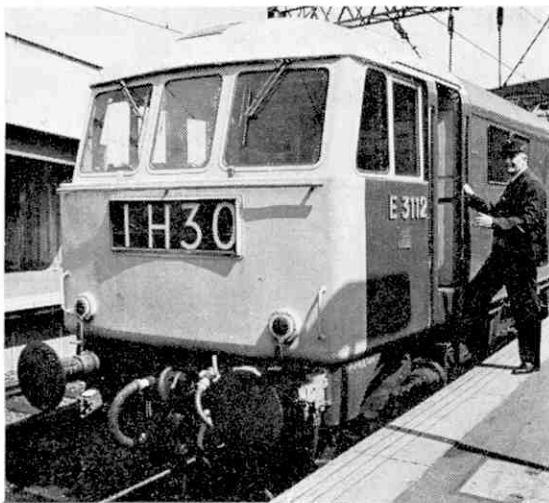
Above, cab end of a new AL6 type electric locomotive, which provide motive power for all the new services. 100 m.p.h. speeds are everyday occurrences. At right, this Manchester suburban train is a far cry from the steam services of not so long ago.
