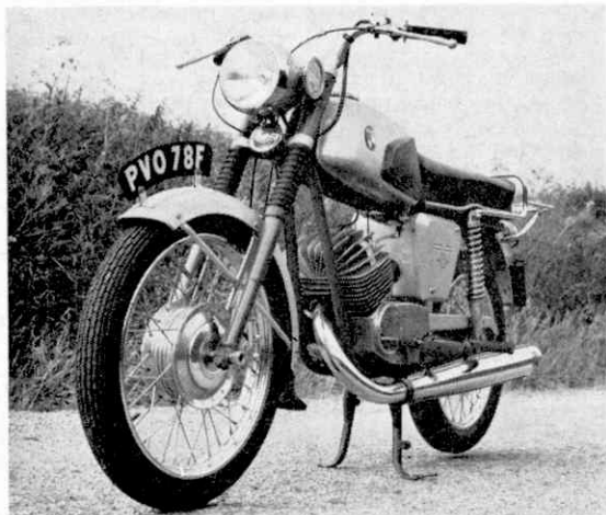
Above: Freedom from ugly wiring is evident, particularly on the engine unit. Note the large cooling fins.
