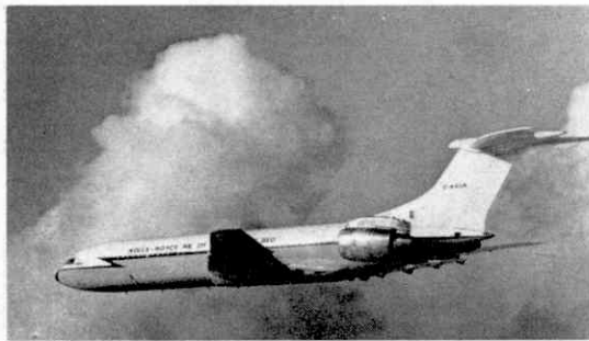
A V.C.10, flying testbed for the Rolls-Royce R.B.211 engine fitted in TriStar "pod".
