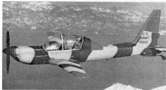
Designated the YO-3A, the aircraft has been adapted from the Schweizer SGS 2-32 glider. Because the glider had a large wingspan of 57 ft. it is possible to keep it aloft on long flights with the aid of relatively little engine power. So Lockheed added a six-cylinder piston engine with a six-bladed propeller. The result a 30 ft. long two-seater aircraft which is inherently quiet.
