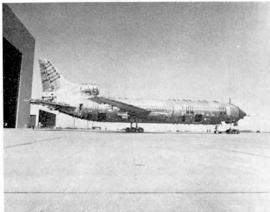
Left: This TriStar will never fly, but it will ensure that airframe stress damage is never likely to endanger its flying sisters.
