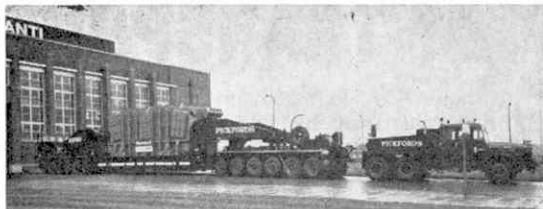
Left, a Scammell Contractor tractor with a 300-ton nett load capacity trailer carrying a 185-ton transformer.
