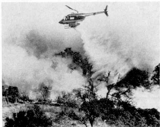
Above, this 204B of Los Angeles C.F.D. is a veteran fire-fighter; it is capable of water drops of more than 300 gallons.
