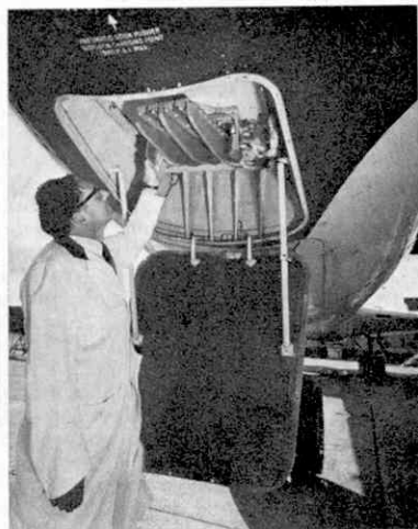
Below, Marconi Doppler navigation aerial in a Super VC10. All BOAC aircraft now have this system.
