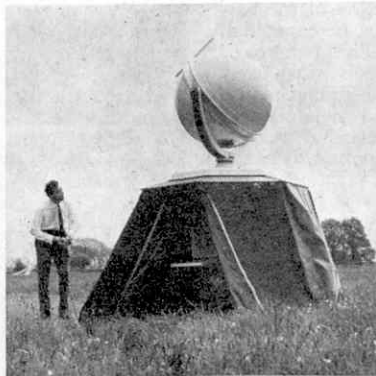
WF-3 X-band automatic tracking wind-finding radar by Plessey is a great aid for meteorologists.
