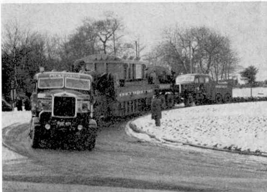
Largest load at time of writing on British roads was this 270 ton transformer on its 85 ton transporter.
