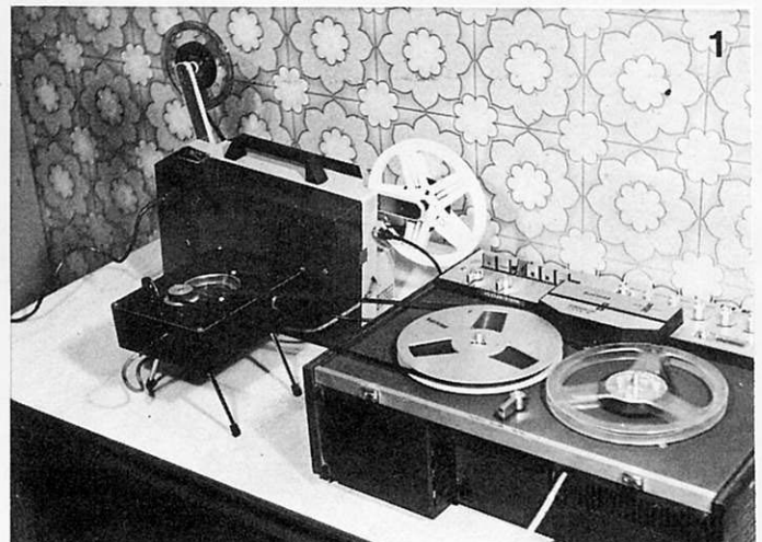
Fig. 1, the Synchrodek – a mechanical/electrical synchroniser for linking projector and recorder – hooked up for operation. The tape from the recorder is looped round the drive capstan of the Synchrodek and a flexible drive is connected to the drive shaft of the projector.
