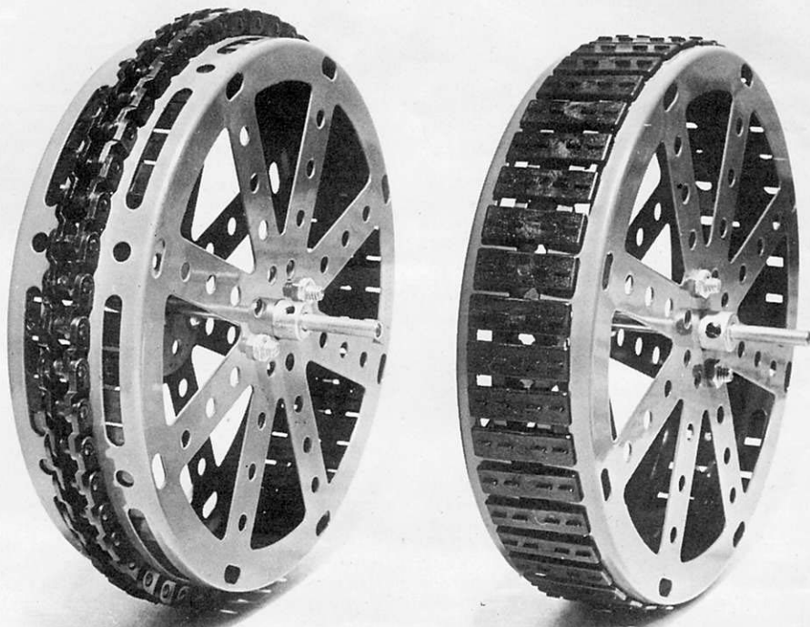
Two examples illustrating the unorthodox use of Meccano Crawler Track, both suggested by Mr. Melvyn Down of Harlow, Essex. Right shows the Track sandwiched, track plates outwards, between two Hub Discs to give a tyred road wheel appearance for models such as Traction Engines; Left shows the Track sandwiched, with track links inwards, to produce a large diameter gear wheel.
