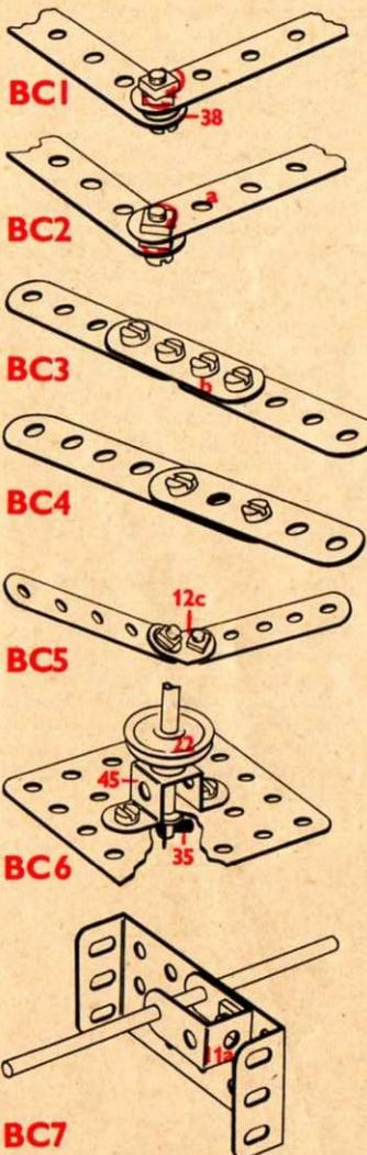
**BC1** is a method of joining two Strips together so that they can move in relation to each other. It is known as 'lock-nutting' and makes use of two nuts tightened together on the bolt. The nuts must not grip the Strips tightly.
