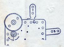
The motor will drive a large number of the smaller models without extra gearing. This diagram shows how extra gears may be added when more power is required. The wheel mounted on the driving-spindle is the  $\frac{1}{2}$  Meccano pinion; the wheel engaged by the pinion is the Meccano 56 toothed gear.
